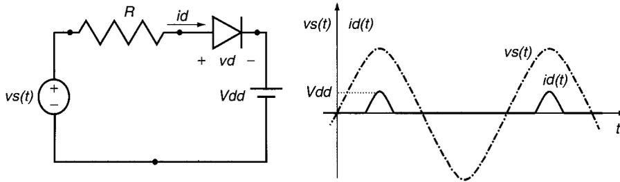
FIGURE 5.5 A Simple Rectifier Circuit with an Ideal Diode: The steady-state solution can be found graphically.
