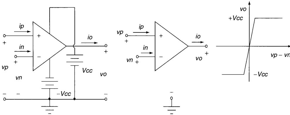
FIGURE 5.3 Multiterminal Nonlinear Circuit Element: An Op-Amp with Five Terminals, its Simplified Circuit Symbol, and an Ideal Characteristic
