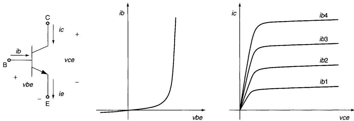
FIGURE 5.2 Three-Terminal Nonlinear Resistive Element: A Circuit Symbol and Characteristics of an  $n$ - $p$ - $n$  Bipolar Junction Transistor
